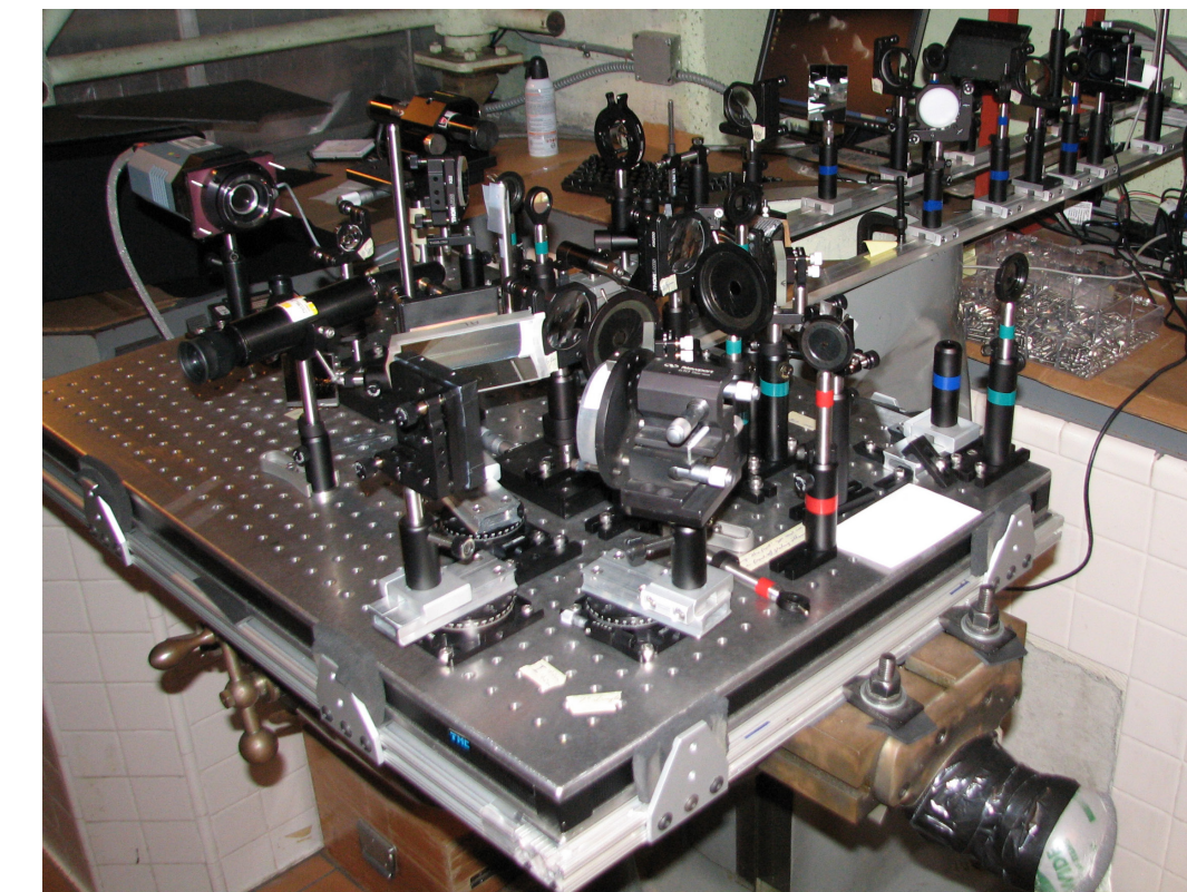
(BELOW) The Tunable Heterodyne Spectrometer being built. (LEFT) Sonia Hosseini, an astronomy graduate student at UC Davis, working on her instrument for the Shane Telescope.
